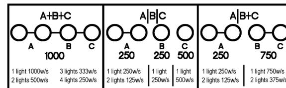
Divide watt-seconds by 2 when using half power (-1 stop).
