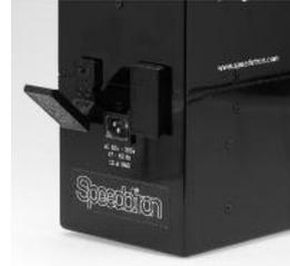
A plastic strip is placed between one end of the Juice Box and the Power Pack to prevent the system from being turned on and running down the battery if it encounters rough handling during shipping.
